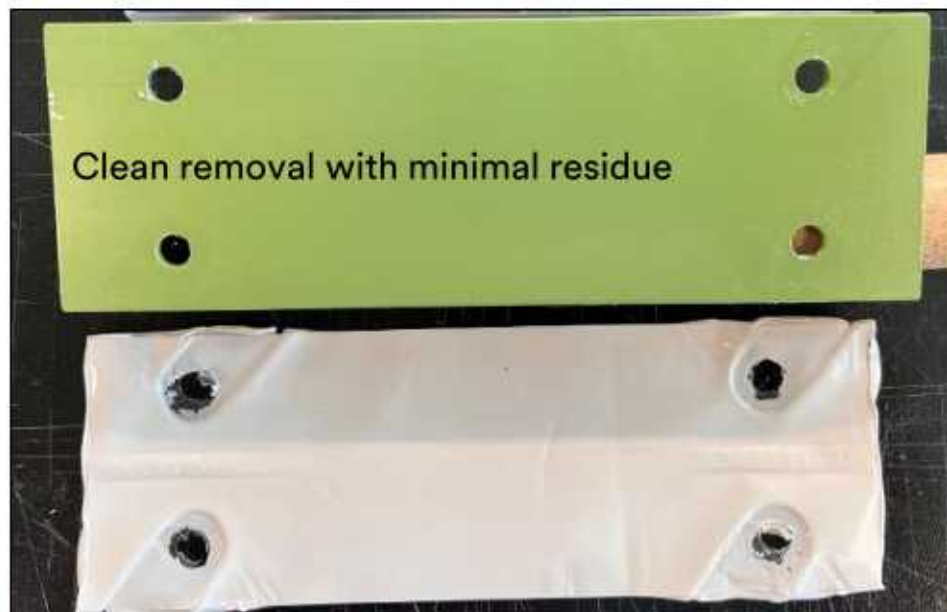
9143FR removed from beam surface
