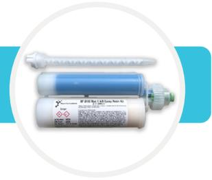
RF 6110 is a two-part volume dispensing structural adhesive system. Designed to cure at room temperature, it is also capable of elevated curing. When cured at room temperature, RF 6110 will provide a glass transition temperature of 108°C and will not produce an amine blush. RF 6110 will provide floating roller bell peel values of 32 pounds per inch, and structural lap shear properties exceeding 4800 psi at room temperature, and above 2100 psi when tested at 220°F.
